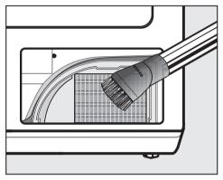
Vacuum up any soiling carefully using a vacuum cleaner dusting brush or small crevice nozzle.
